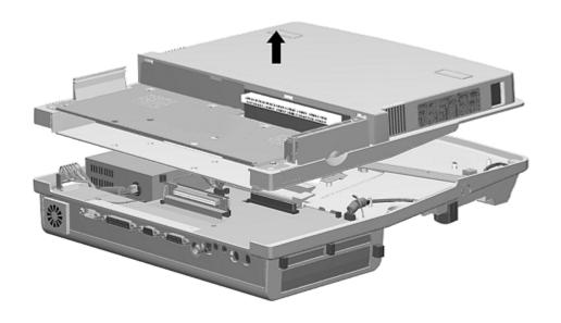
Figure 7-12. Removing the Bottom Cover
